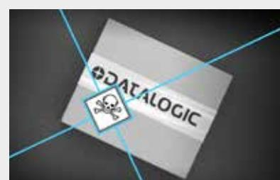
The PST is not just a tool for item sorting. The algorithm can be used for many different purposes and applications. For instance it can detect the presence of stickers or logos as well as identify items by means of the artworks printed on the package.
