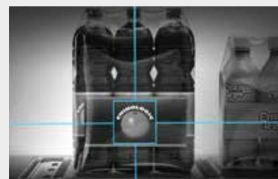
Thanks to its capability to manage big databases of patterns, the PST is able to distinguish among thousands of different items manufactured or simply conveyed on the same line. The algorithm delivers robust recognition in any situation (e.g. 360° pattern rotations, perspective distortions, different scales and light variations).
